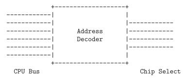
The Chip Select registers must be programmed such that they match the linkcmds settings. In the gen68340 BSP, ROM and RAM addresses can be found in both the linkcmds and initialization code, but this is not a great way to do this. It is better to define addresses in the linker script.
